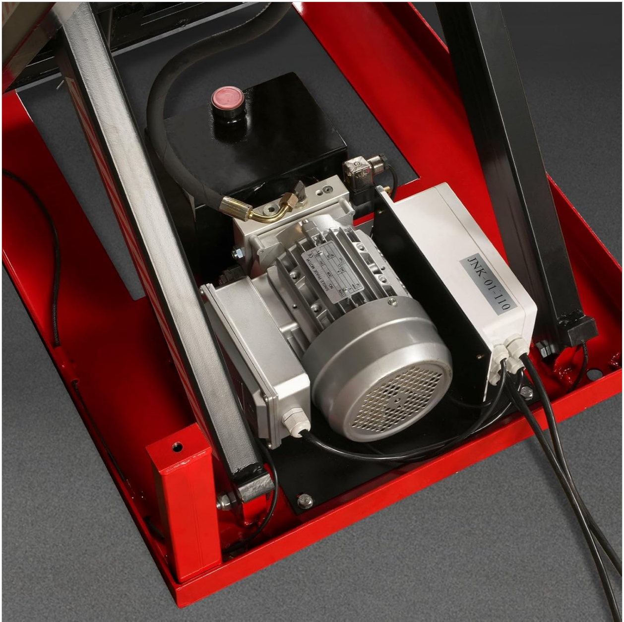
Figure 6.2: Detailed view of the hydraulic pump and motor assembly, responsible for the lifting mechanism.
