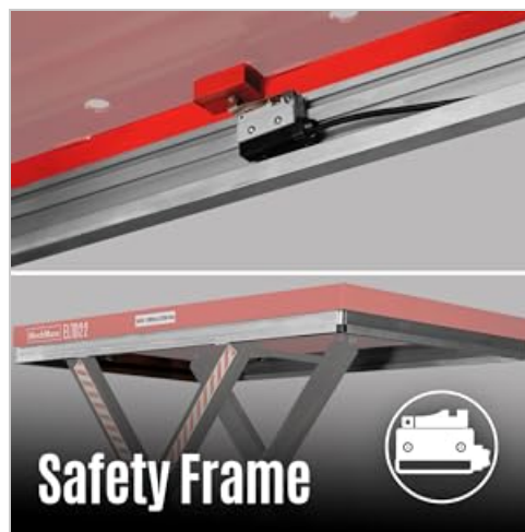
Figure 6.4: The safety frame located beneath the platform, designed to detect obstructions and prevent crushing during descent.
