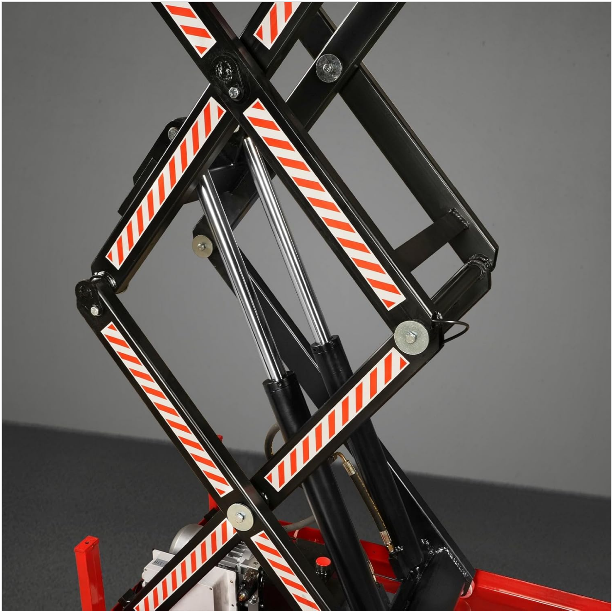
Figure 6.3: Close-up of the robust double scissor mechanism and hydraulic cylinders that provide stable and powerful lifting.
