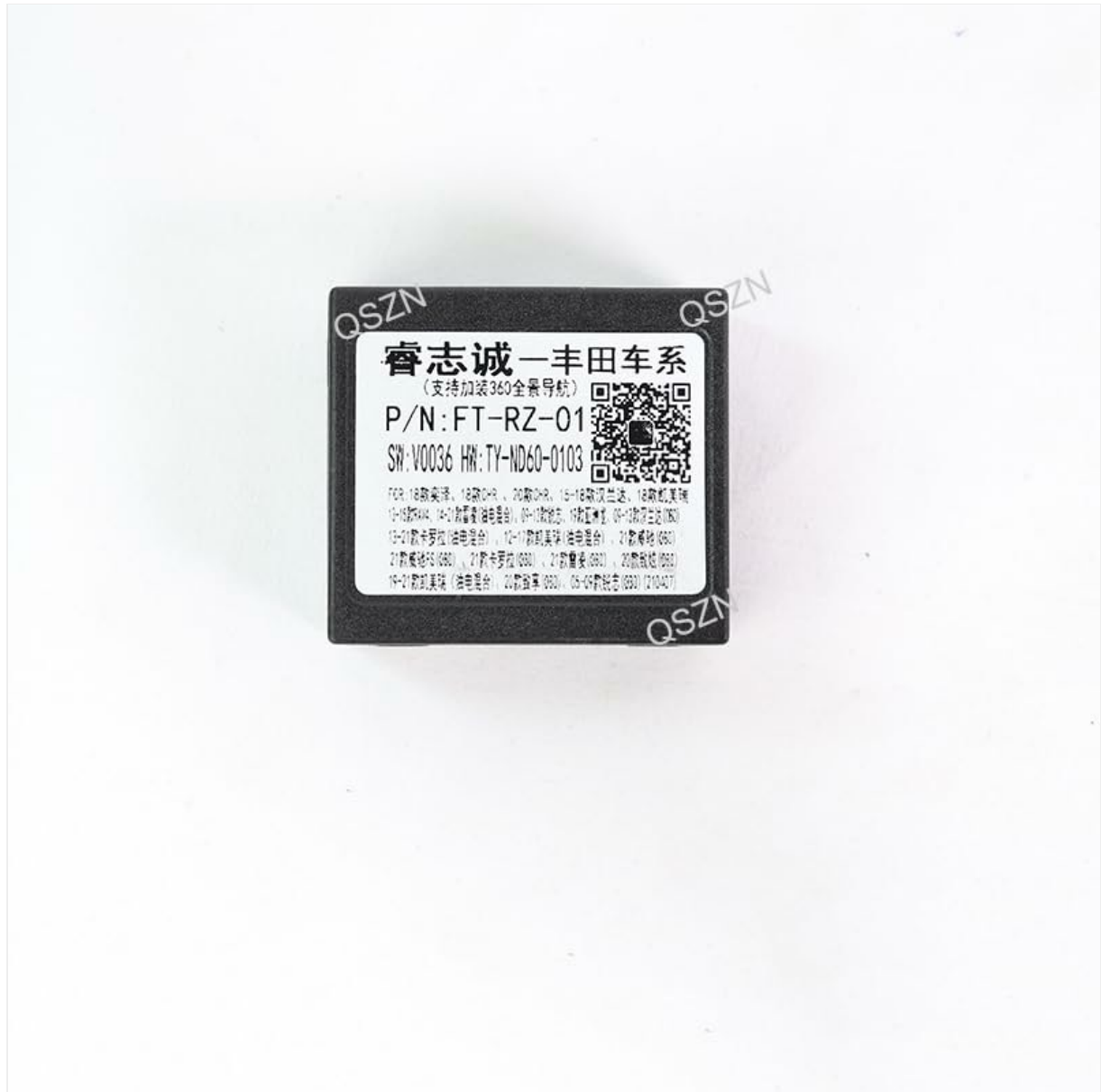
Image 3.1: The FT-RZ-01 Canbus Box module. This compact black box processes CAN-bus signals. It features a label with product information and a QR code. For more information, scan the QR code or visit
