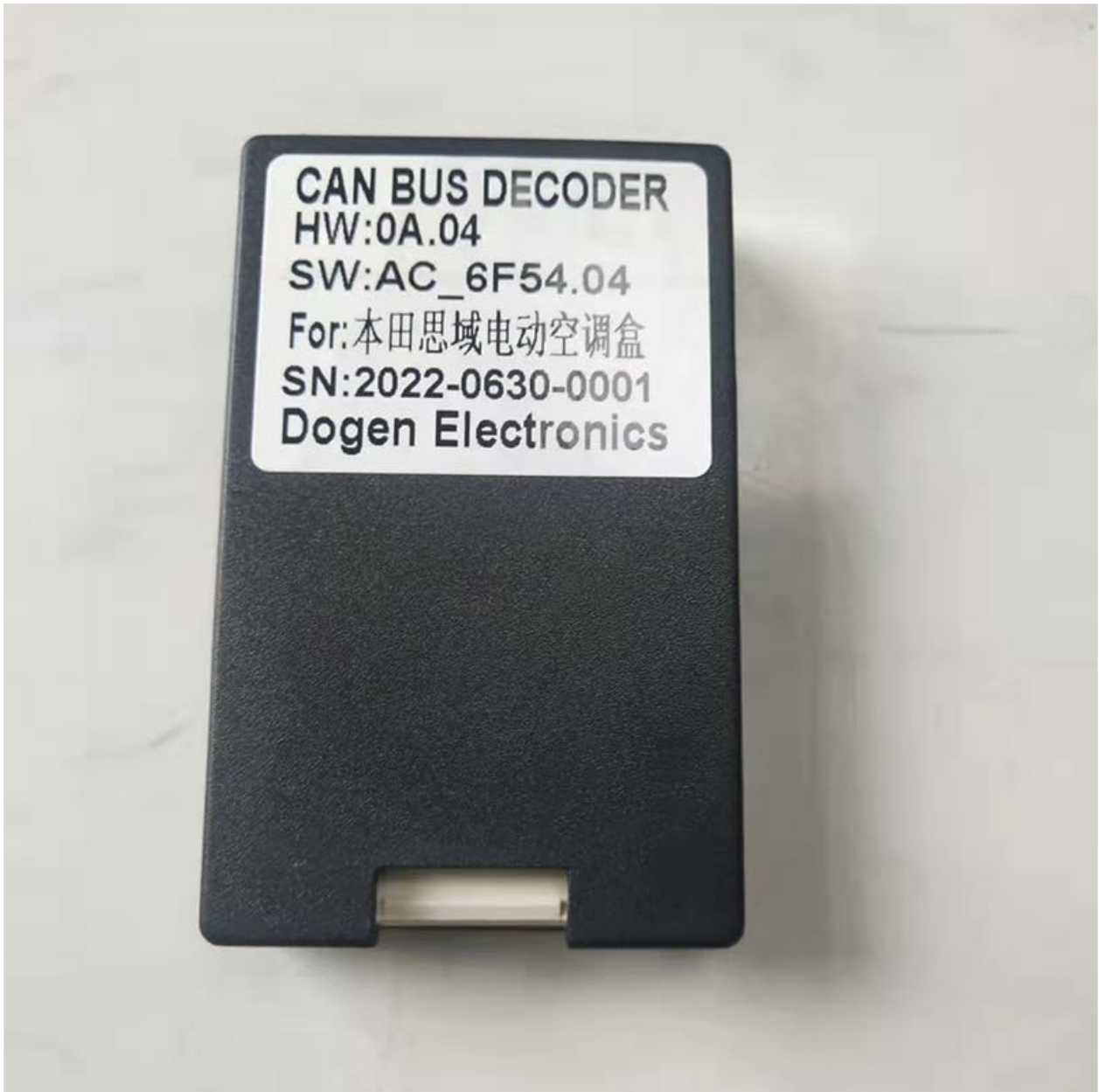
Figure 2: The Canbus Box Adaptor, showing its label with model and serial information.
