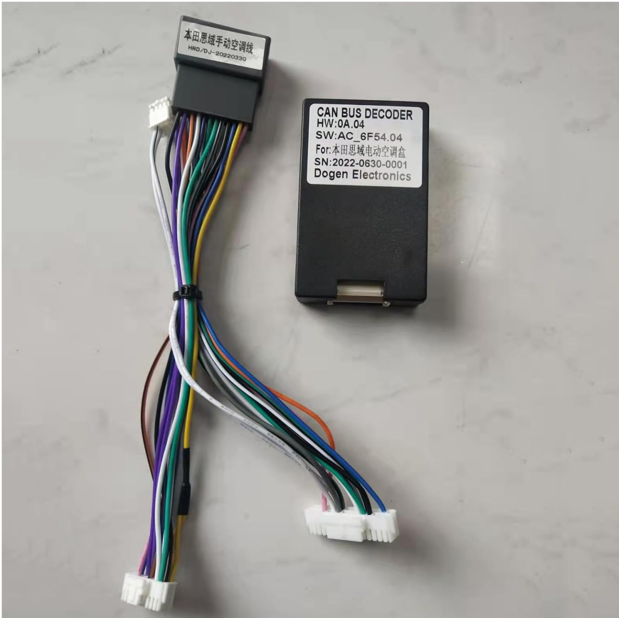
Figure 1: The complete package includes the Canbus Box Adaptor and its associated multi-pin wiring harness.
