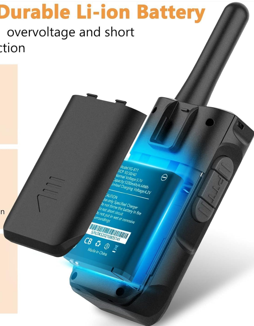
Image 5.1: Battery Installation and Safety. This image illustrates how to insert the 1200mAh Li-ion battery and highlights its safety features like overcharge protection and IEC62133 certification.
