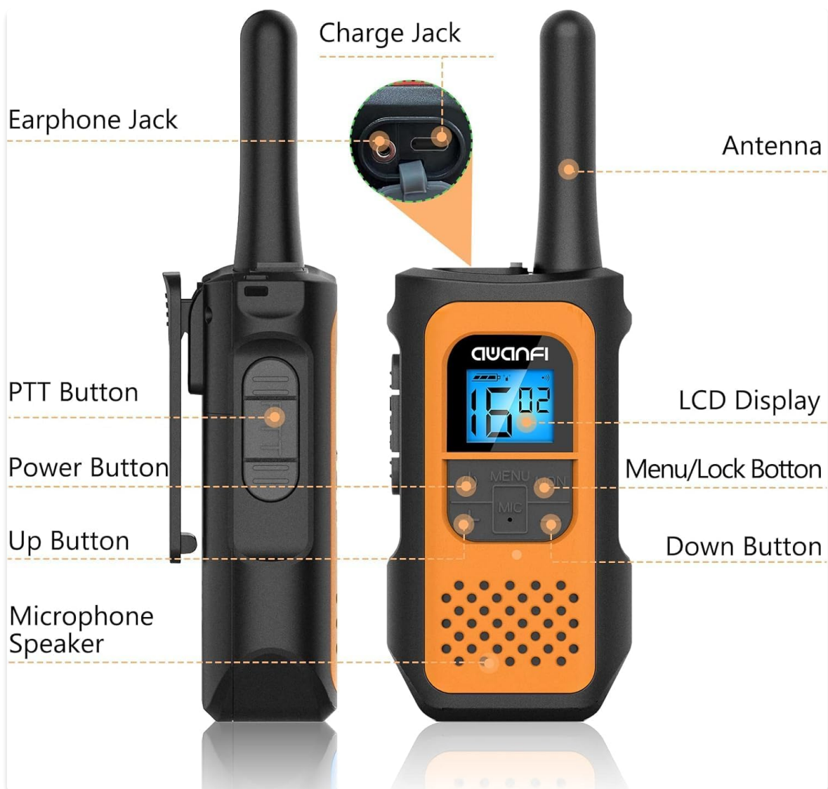
Image 4.1: AWANFI YG-811 Component Diagram. This image labels the antenna, earphone jack, charge jack, PTT button, power button, microphone/speaker, LCD display, menu/lock button, up button, and down button.
