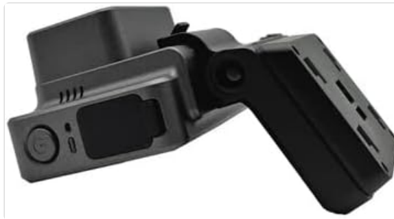
Image: Side view of the dash cam, showing the adjustable mounting bracket.
