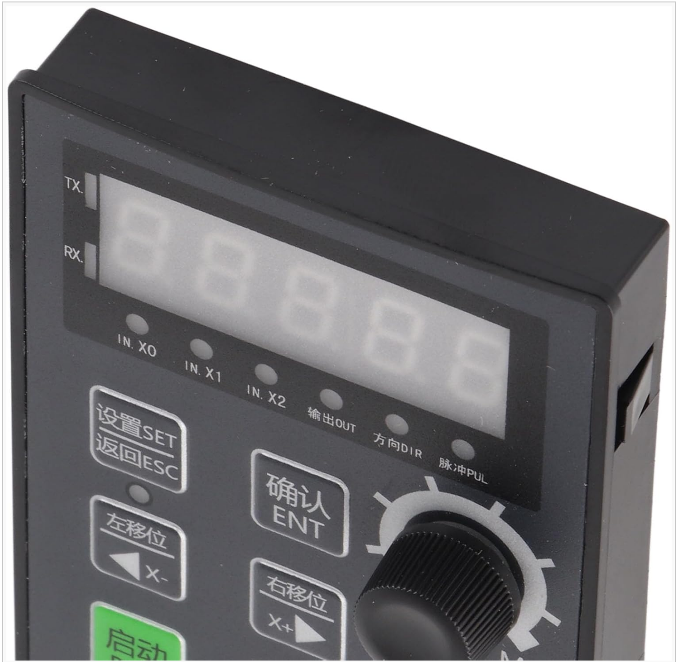
Figure 5: Detailed view of the 5-digit digital display and status indicators (IN.X0, IN.X1, IN.X2, OUTPUT, DIR, PUL).
