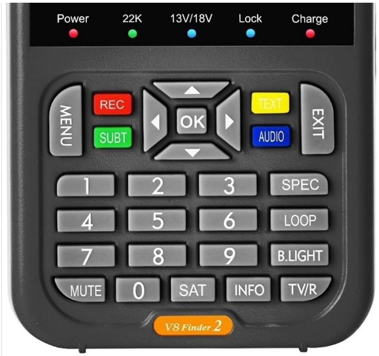
Figure 4.1: Front view of the SURRYN V8 Finder2, showing the 3.5-inch LCD screen, menu icons, and control buttons. Key indicators for Power, 22K, 13V/18V, Lock, and Charge are visible below the screen.
