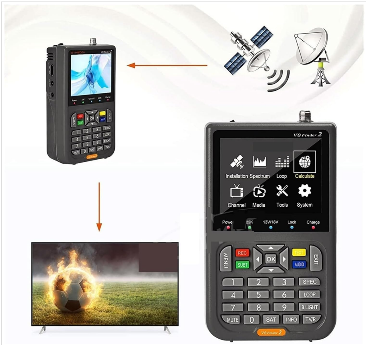
Figure 5.2: Diagram illustrating the connection of the V8 Finder2 to a satellite dish and subsequently to a television for signal display.
