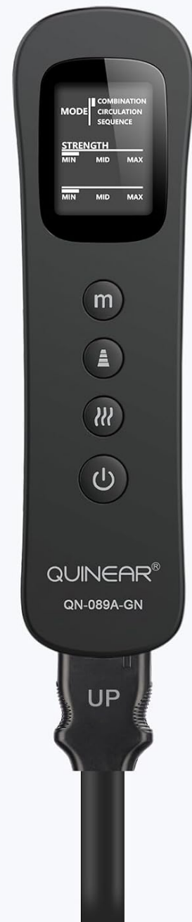
Figure 5: Handheld controller with buttons for On/Off, Heat, Mode, and Air Pressure.
