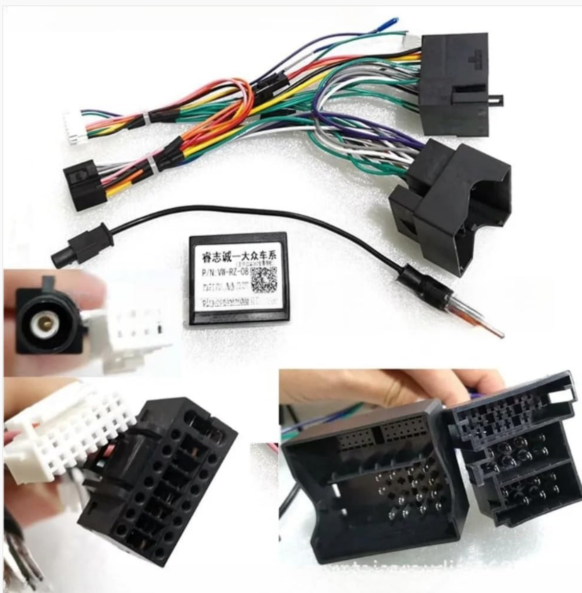
Image 1: The XIBEIKE VW-RZ-08 Canbus Box, a compact black module with a label indicating part number VW-RZ-08.
