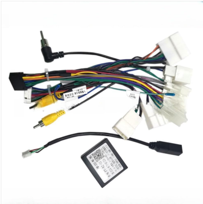
Figure 3: The wiring harness assembly including the integrated CANbus box. The CANbus box is a critical component for translating vehicle data signals for the aftermarket radio, enabling features like steering wheel control integration.
