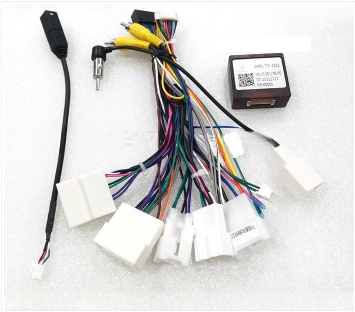
Figure 2.1: Overview of the XIBEIKE RP5-TY-101 Canbus Box and Wiring Harness components. This image displays the main Canbus decoder box, the multi-pin wiring harness with various connectors, and an antenna adapter cable.
