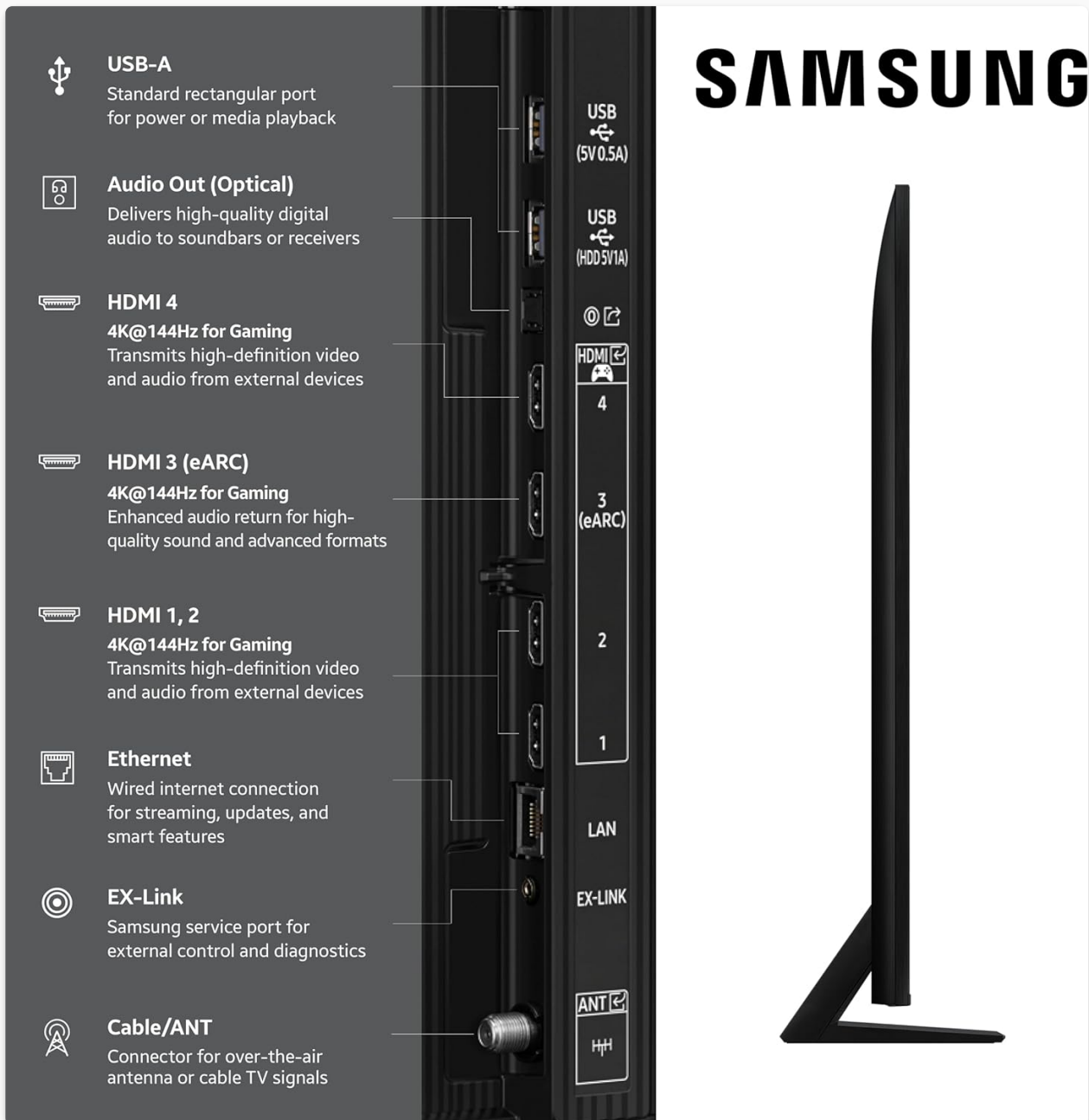
Figure 2.2: Rear panel connections for the Samsung QN80F TV.
