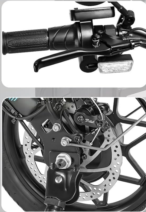
Figure 5.4: A detailed view of the mechanical disc brakes, highlighting the 2-piston system designed for fast and effective braking.
