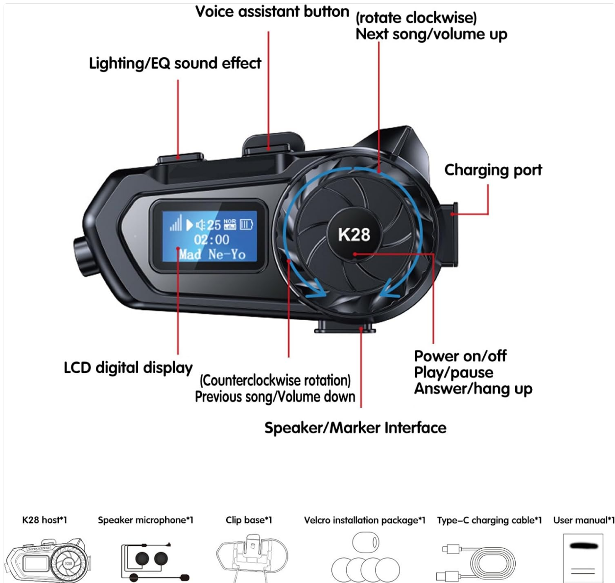
Image 4.1: Bluetooth Unit Controls and Package Contents. This image illustrates the various controls on the K28 Bluetooth unit and lists the components included in the package, such as the K28 host, speaker microphone, clip base, Velcro installation package, Type-C charging cable, and user manual.
