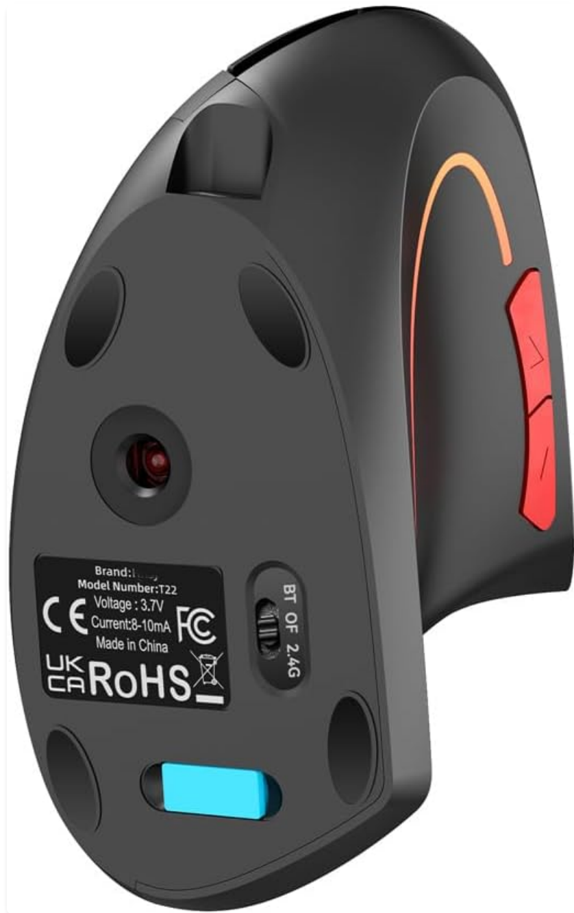
Image: The underside of the T22 Vertical Mouse, showing the optical sensor, product labels, and the switch for selecting between Bluetooth and 2.4G wireless modes.
