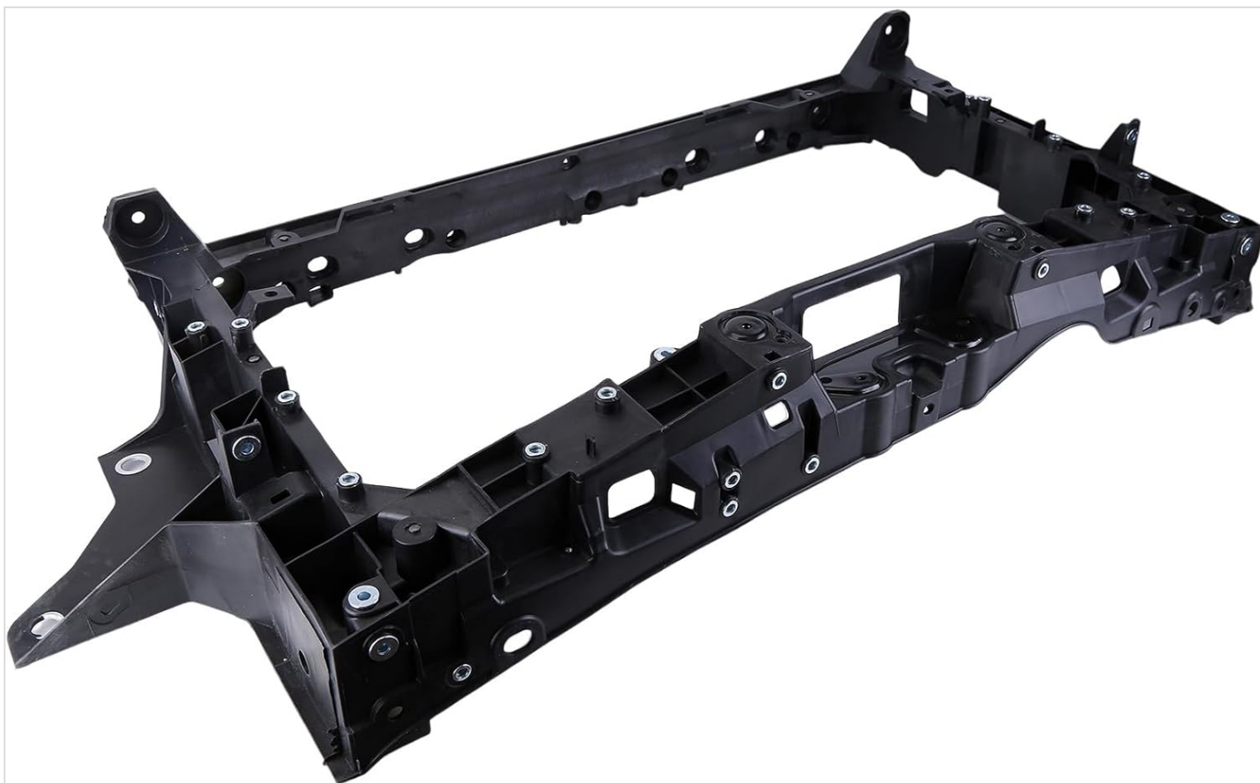
Image 2: Angled view of the radiator support assembly, providing a perspective of its three-dimensional form and various attachment points.
