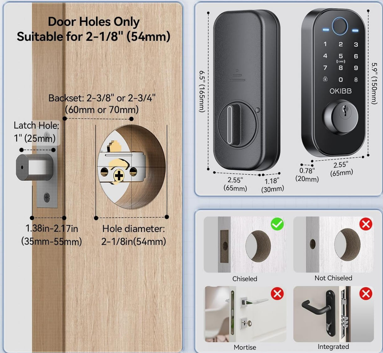
Image 4.1: A detailed diagram illustrating the required door hole diameter (2-1/8" or 54mm), backset (2-3/8" or 60mm, or 2-3/4" or 70mm), and latch hole (1" or 25mm) for proper installation.
