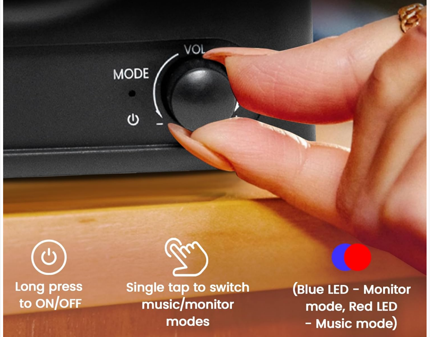
Image: Multifunction knob for power, volume, and mode.
