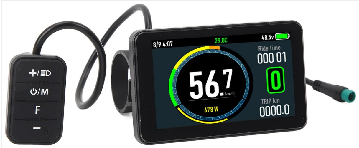
Image: The T8 display screen showing various metrics including speed, battery level, voltage, ride time, trip distance, power, and temperature.
