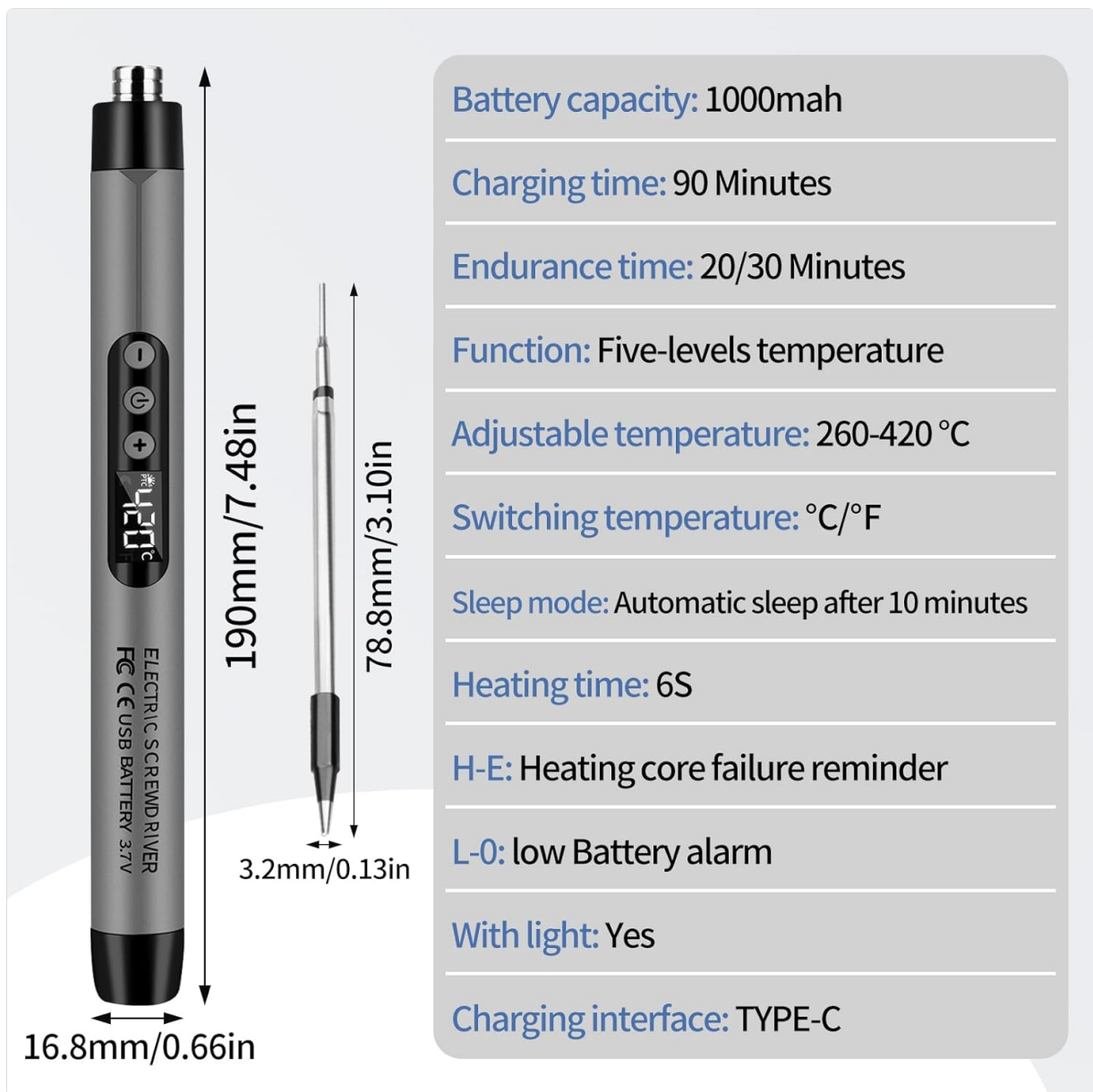
Figure 10: Visual representation of the soldering iron's dimensions and a summary of its key specifications.
