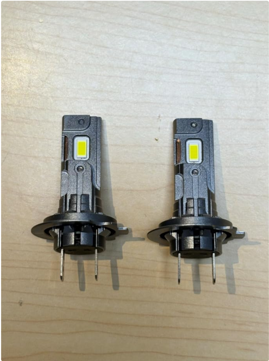
Image: A close-up view of two Termitor H7/H7LL LED fog light bulbs, showing their compact design and LED chips.
