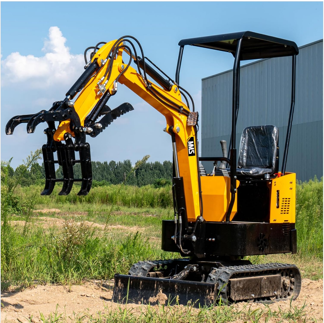
Image 6.1: Grapple in Operation. This image shows the MMS Mini Excavator Grapple Attachment mounted on a mini excavator, ready for operation in an outdoor setting.
