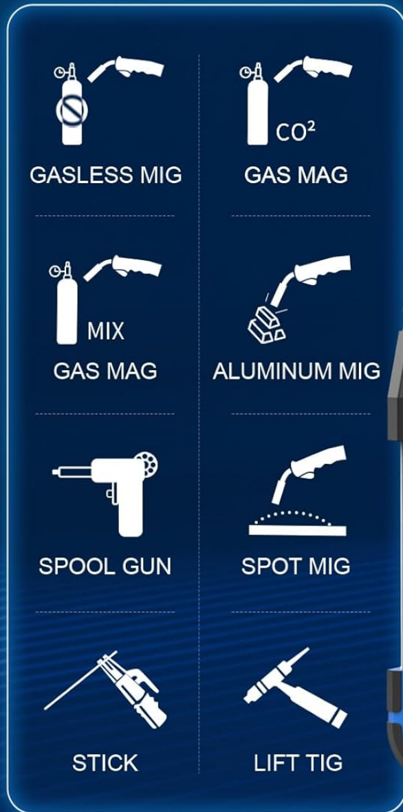
Figure 8: The 8-in-1 multi-process capabilities of the welder.
