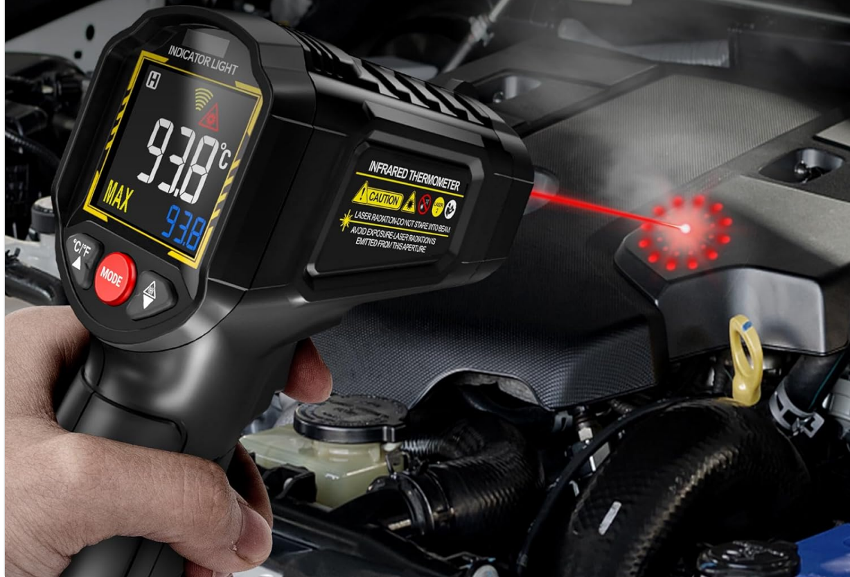
Figure 7: Using the TH203 for overheating detection in an automotive application.
