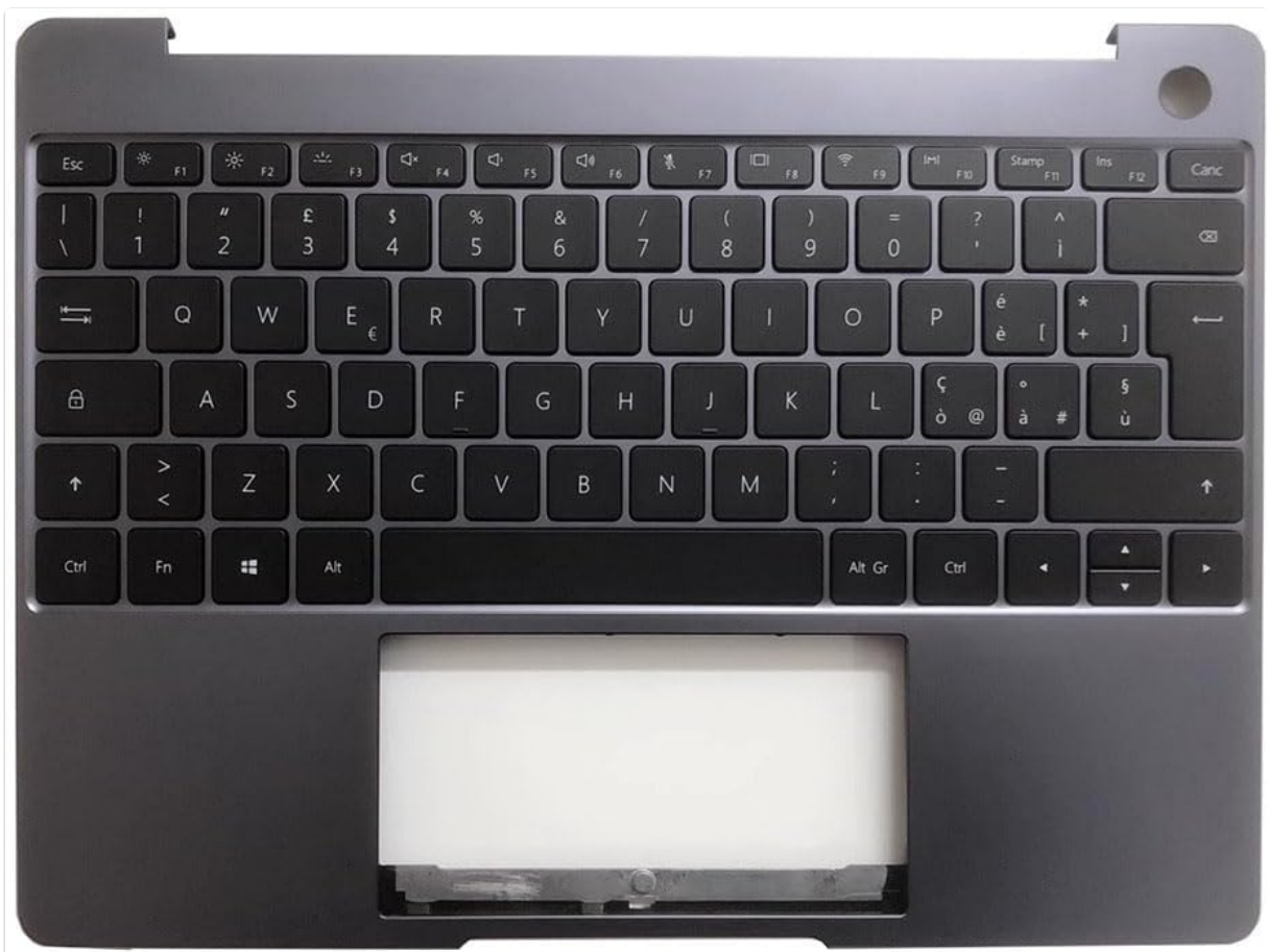
Image: Huawei Matebook 13 Replacement Palm Rest and Italian Keyboard Assembly. This image displays the complete upper case component, including the integrated Italian layout keyboard and the touchpad cutout.
