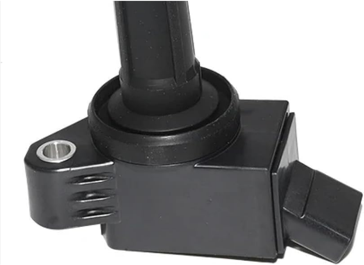
Figure 4: Bottom view of the ignition coil, showing the boot that connects to the spark plug. Ensure this is clean and free of damage.
