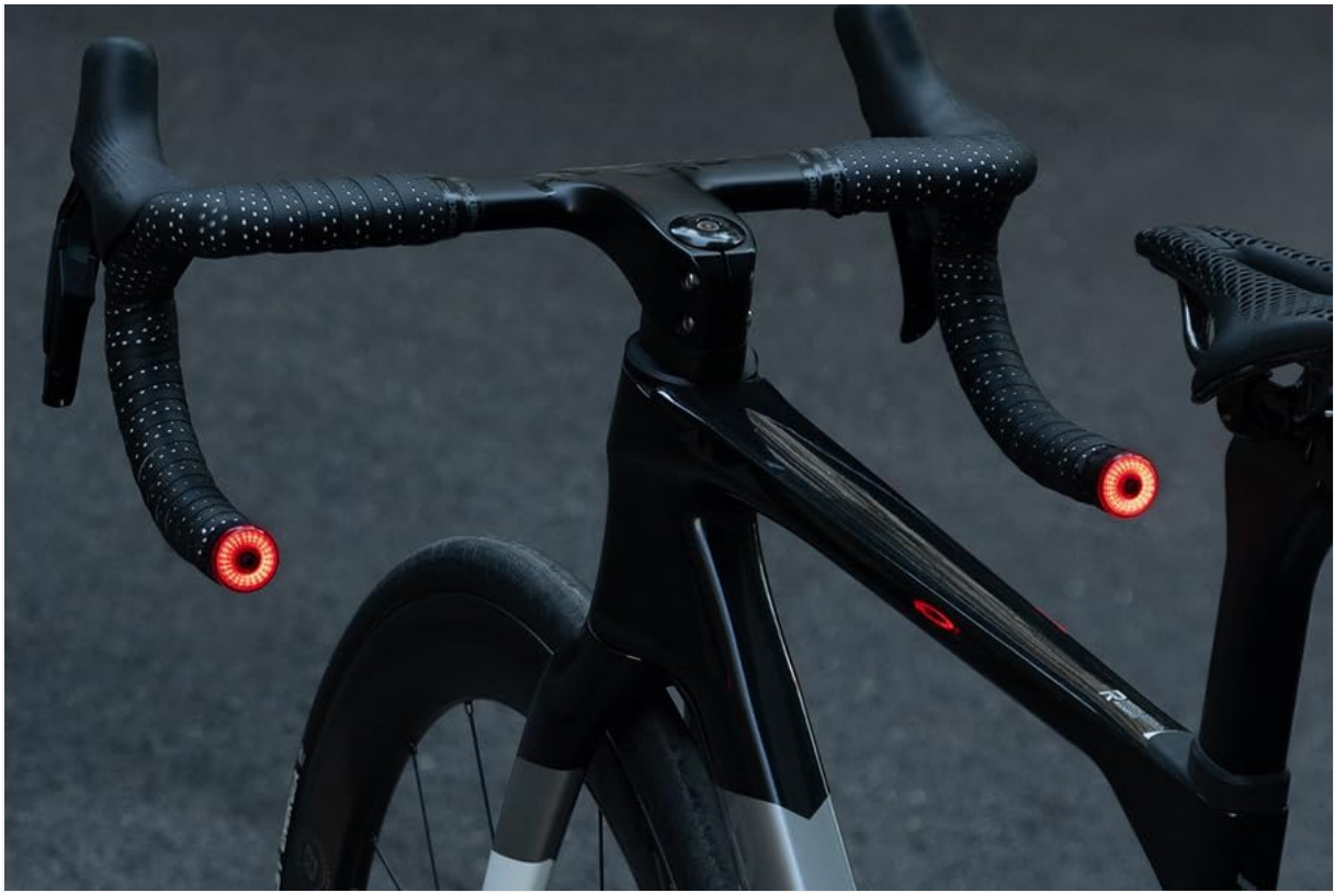
Image 4.2: Both handlebar end lights illuminated on a bicycle, demonstrating their visibility from the rear.
