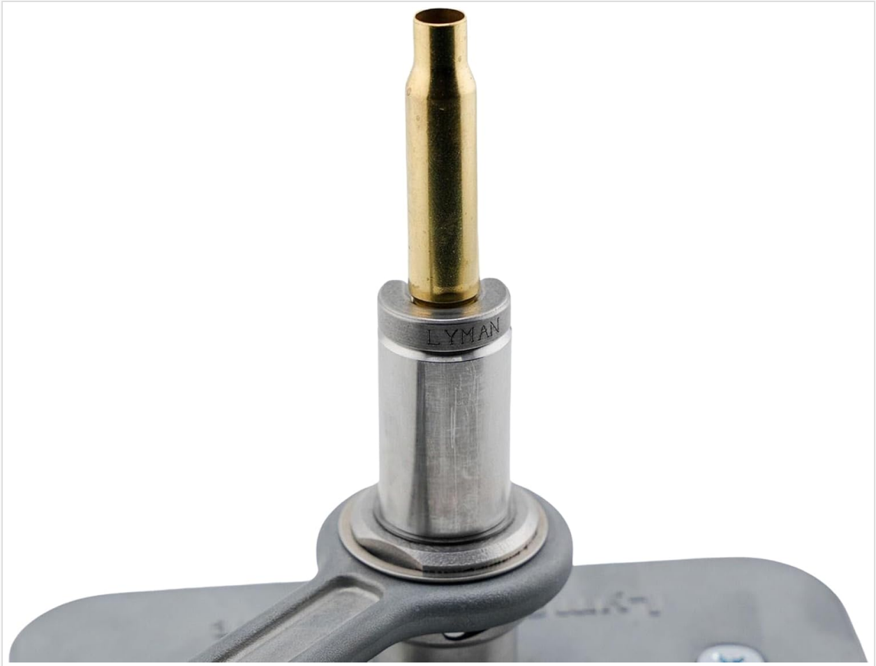
Image: A detailed view of the priming process, showing a brass case being precisely primed by the Accu-Prime tool.
