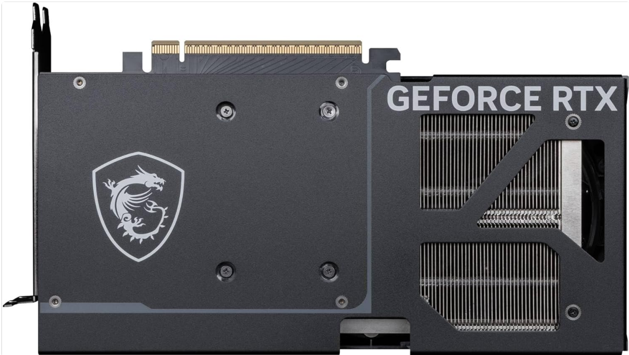
Image: The backplate of the graphics card, which provides structural rigidity and aids in passive cooling. Regular cleaning helps maintain its efficiency.
