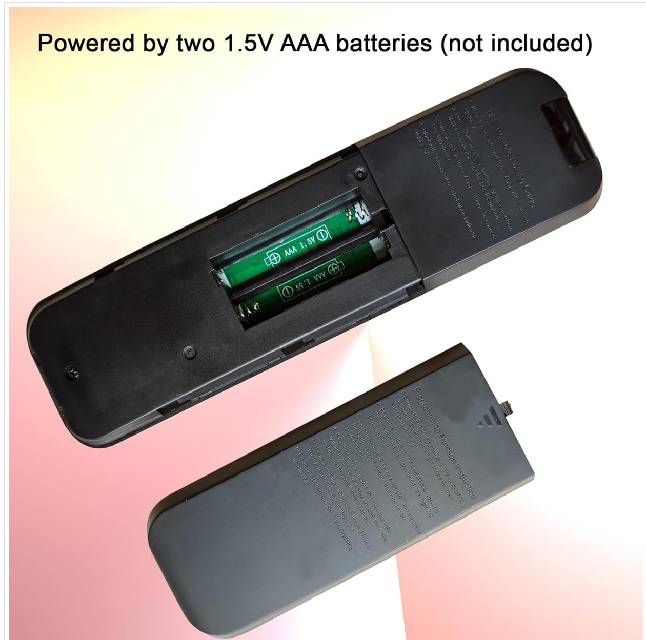
Image 2: View of the RC-200 remote control with the battery compartment open, showing the slots for two 1.5V AAA batteries.
