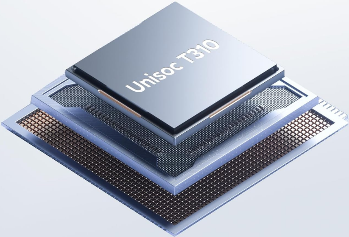
Figure 7.1: Unisoc T310 Processor. This image details the specifications of the Unisoc T310 processor, highlighting its powerful quad-core architecture, 2.0GHz ultimate frequency, and 12nm advanced process technology.
