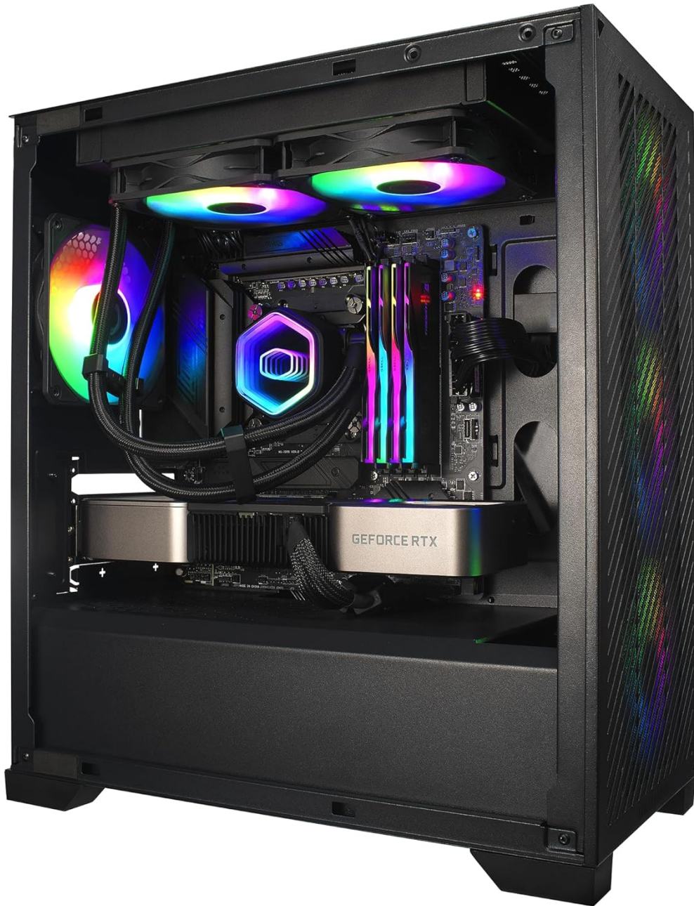
Image 3.2: The liquid cooler fully installed within a computer case, demonstrating proper placement and cable routing.
