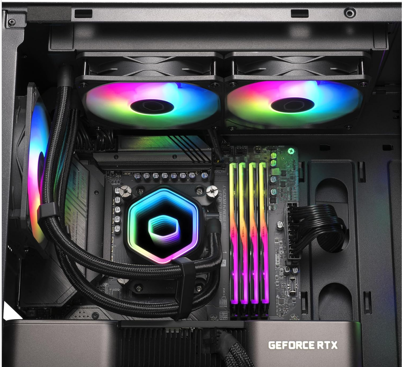
Image 5.1: A top-down view of the cooler installed in a PC case, showing the fans mounted to the radiator and the pump connected to the CPU.
