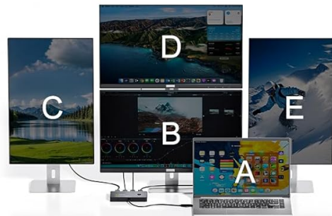
Figure 4: Visual representation of Mirror and Extend display modes.
