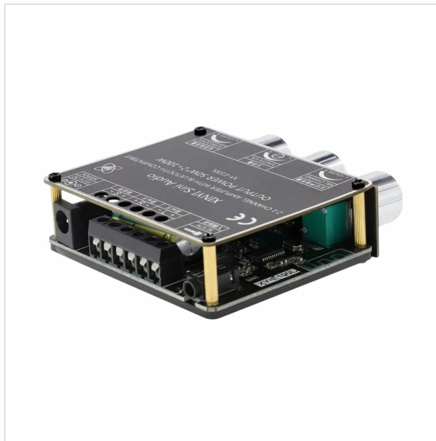
Image: The NONLOTDIO XY-E100L amplifier module. Visible features include the DC power input terminal (DC 9-24V), speaker output terminals for left, right, and subwoofer channels, an AUX input, and a master volume control knob. The board clearly indicates its model number 'XY-E100L' and its 2.1 channel, 50W*2 + 100W output power with Bluetooth compatibility.
