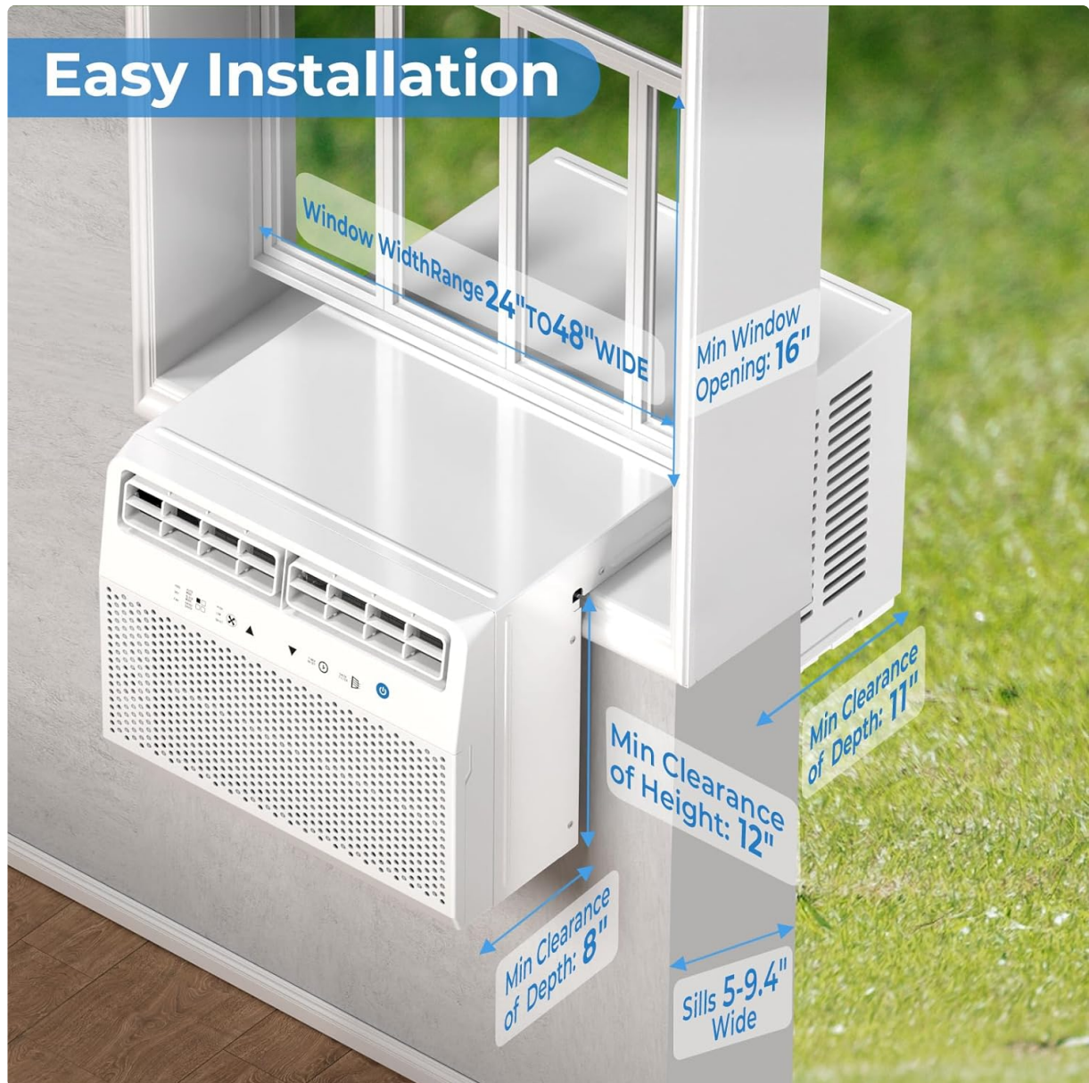
Figure 2: Easy Installation Diagram with Window Dimensions.
