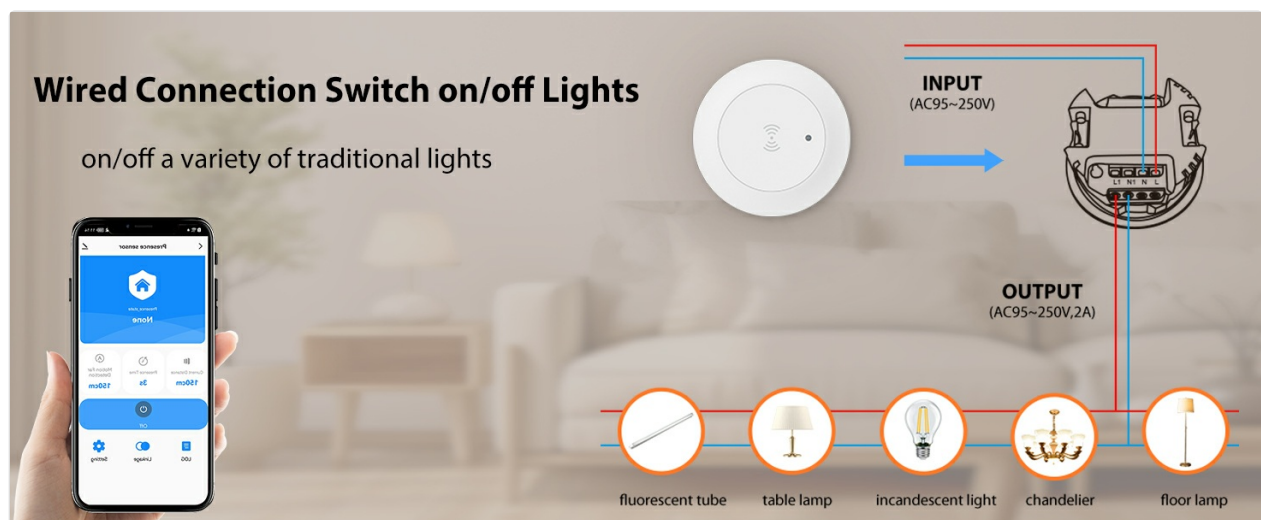
Figure 5.1: Wiring diagram for connecting the sensor to an AC power source and various light fixtures. The diagram illustrates input (AC95-250V) and output (AC95-250V, 2A) terminals, showing connections for fluorescent tubes, table lamps, incandescent lights, chandeliers, and floor lamps.
