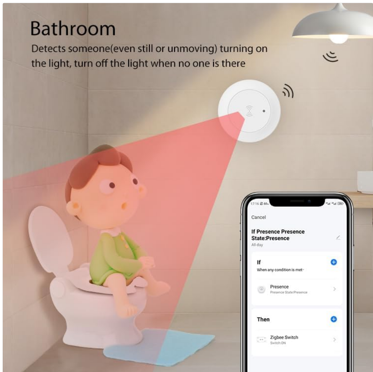
Figure 6.3: Illustration of light automation based on presence and the app setting for presence time delay.
