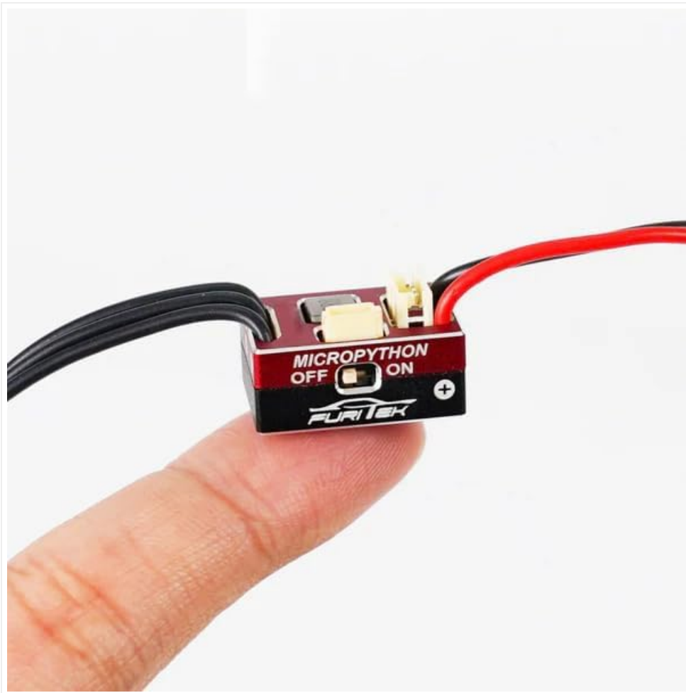
Image: The compact Furitek MicroPython ESC, showing its wire connections.
