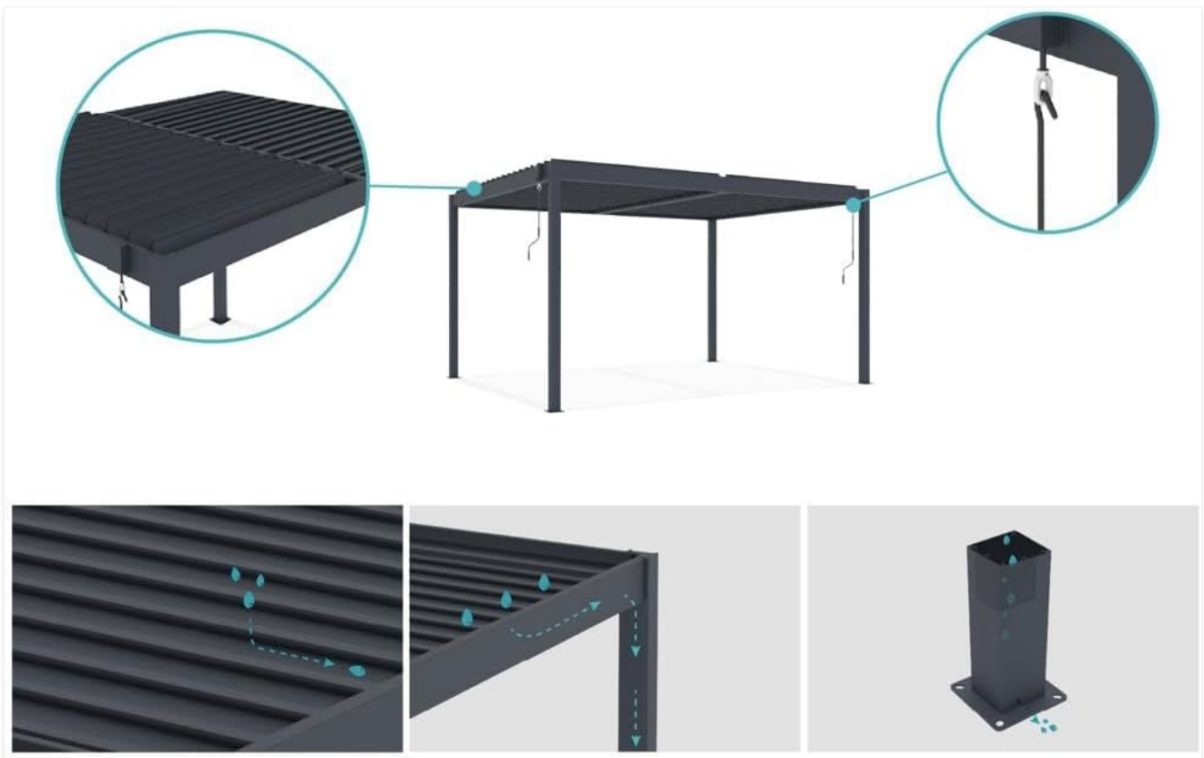
Image 7.1: Diagrams showing how water drains from the louvers into the frame and down the columns.
