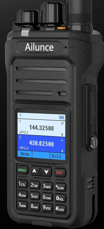
Figure 2.3.2: The Ailunce HA1UV radio highlighting its dual-band capability, operating on both 2m and 70cm frequencies.
