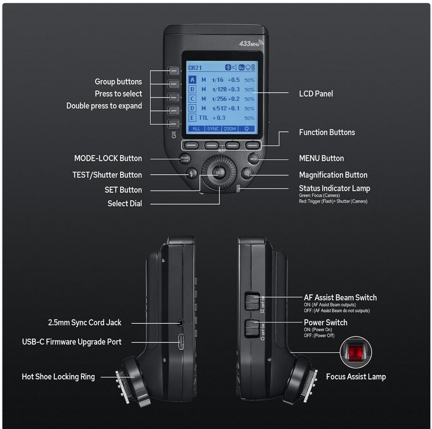
Figure 3: A detailed diagram providing an overview of all physical controls and ports on the FT433N trigger, including the LCD panel, group and function buttons, mode-lock, test/shutter, set button, select dial, AF assist beam, power switch, 2.5mm sync cord jack, USB-C firmware upgrade port, hot shoe locking ring, and focus assist lamp.
