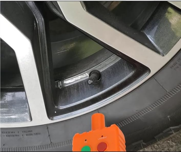
Image 6: Correct positioning of the tool for sensor activation
