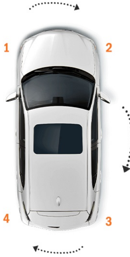
Image 5: Recommended sensor activation sequence
