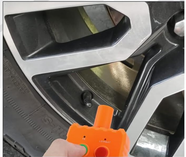
Image 6: Correct positioning of the tool for sensor activation
