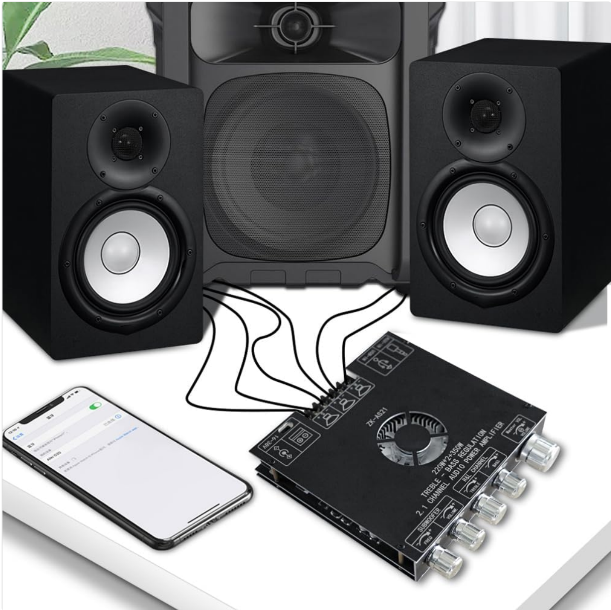
Figure 7.1: An example setup showing the ZK AS21 amplifier board connected to a pair of stereo speakers and a subwoofer, with a smartphone wirelessly streaming audio via Bluetooth.
