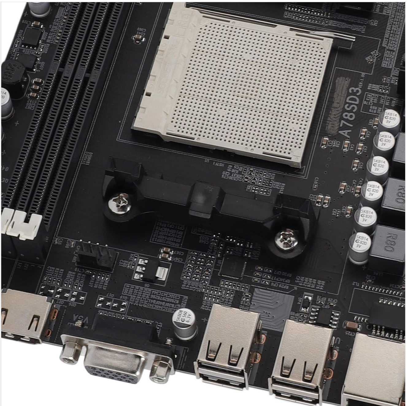
Figure 3.1: Close-up view of the AM3 CPU socket on the Denash A78SD3 Motherboard. This image shows the pin grid array (PGA) socket where the processor is installed.
