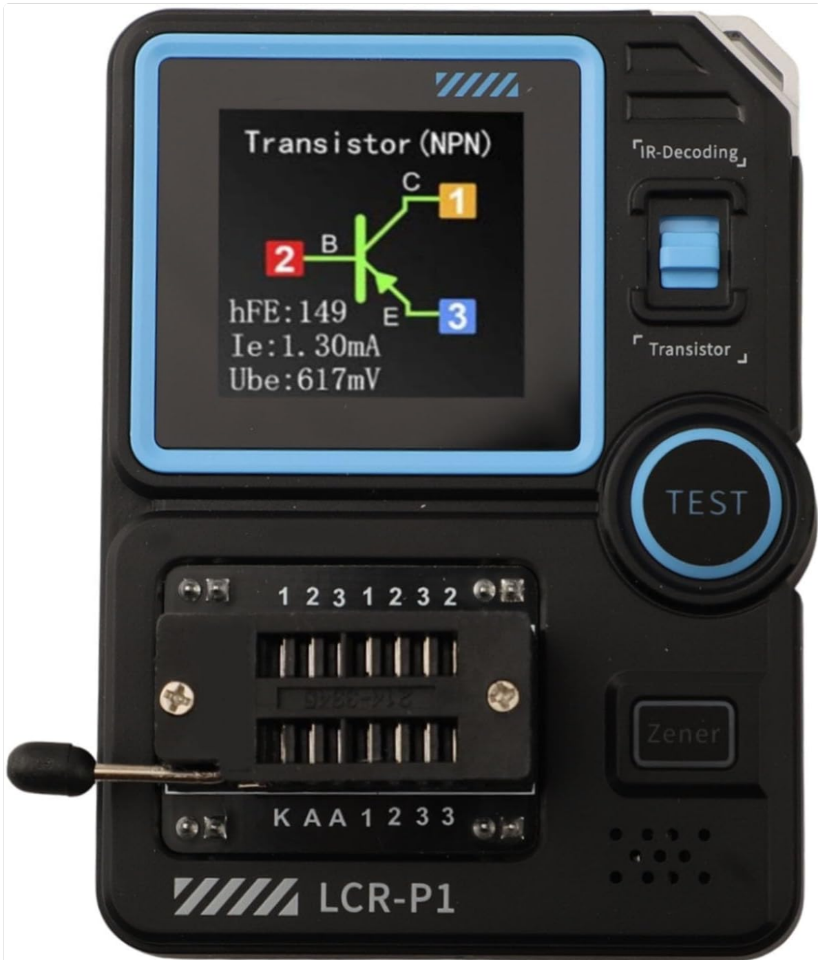
Image 5.1: A close-up of the LCR-P1 tester's screen displaying the results of a transistor test, including NPN type, hFE, collector current (Ic), and base-emitter voltage (Ube).
