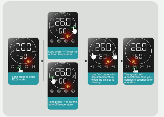
Image: Detailed view of the Premier Smart Controller, explaining ECO Mode, temperature settings, fan speed, light control, and ON/OFF functions.
