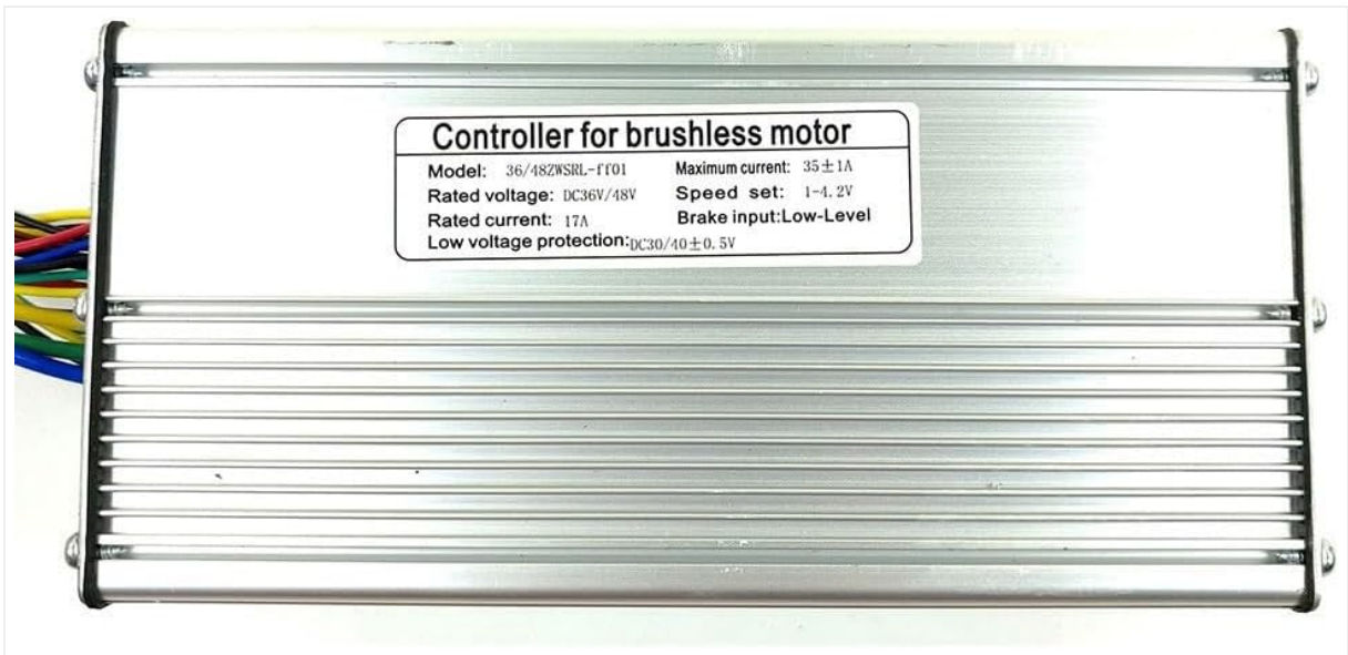
Image 8.1: Controller label displaying key specifications.
