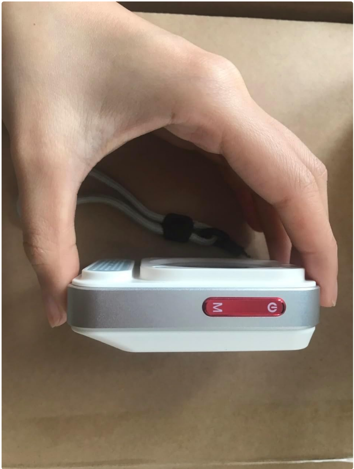
Figure 2.3: Side view of the detector, showing the power and menu buttons.
