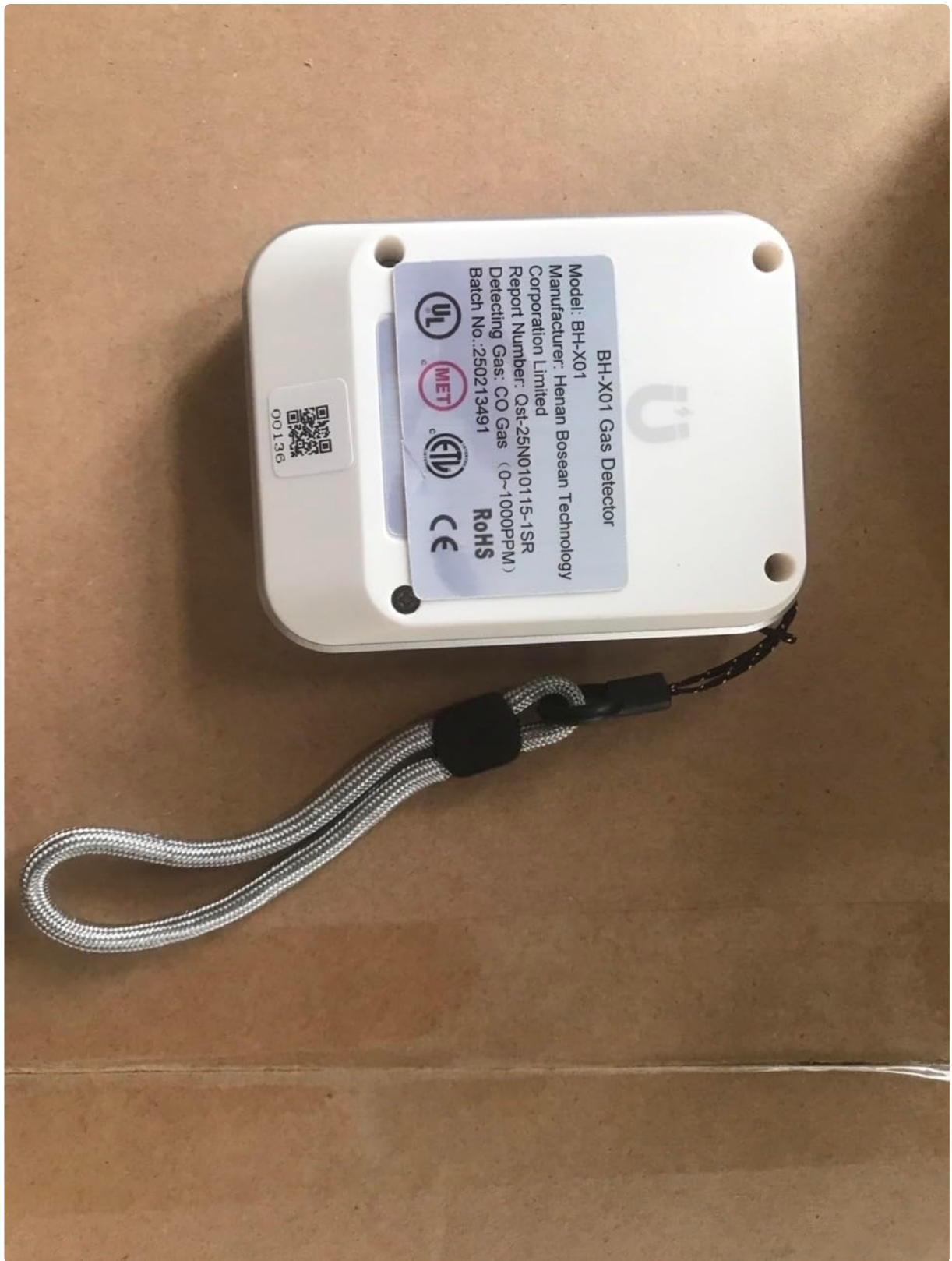
Figure 2.4: Back view of the detector, featuring the product label and magnetic attachment points.
