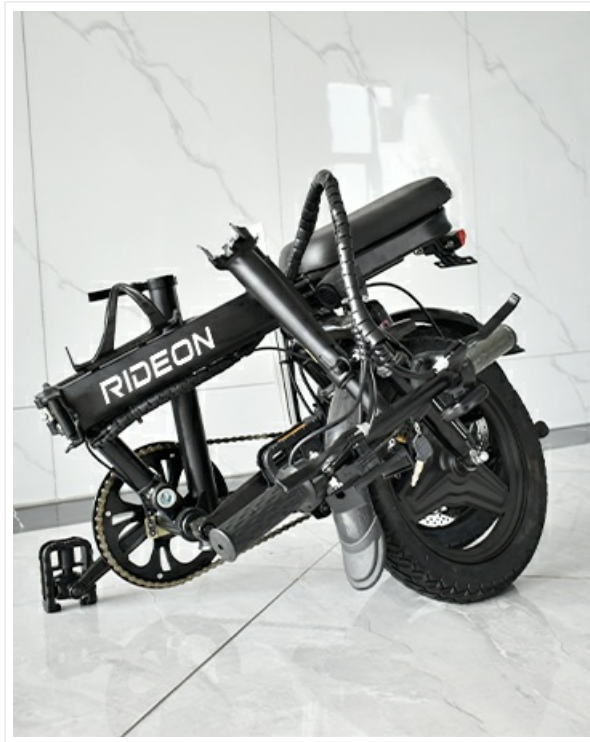
Folding Mechanism: The bike shown in its compact, folded state, demonstrating its portability.
