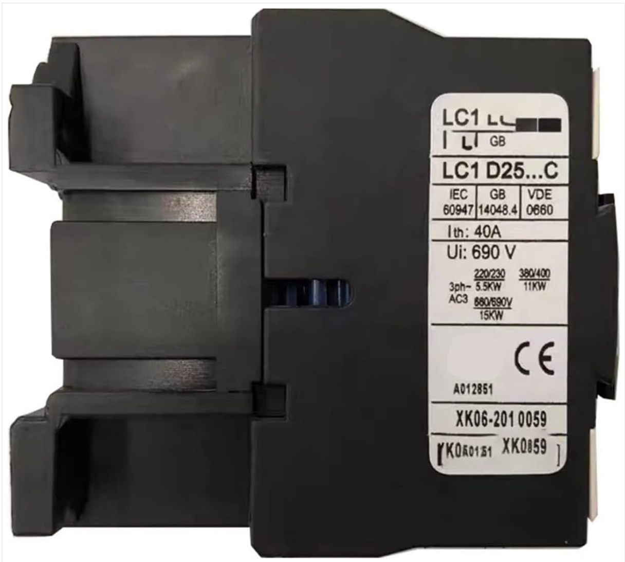
Figure 3.2: Side View with Specifications. This image shows the side of the contactor, highlighting the product label with detailed technical specifications such as IEC, GB, VDE standards, thermal current (I th : 40A), rated insulation voltage (U i : 690V), and power ratings for 3-phase applications (e.g., 5.5kW at 220/230V).
