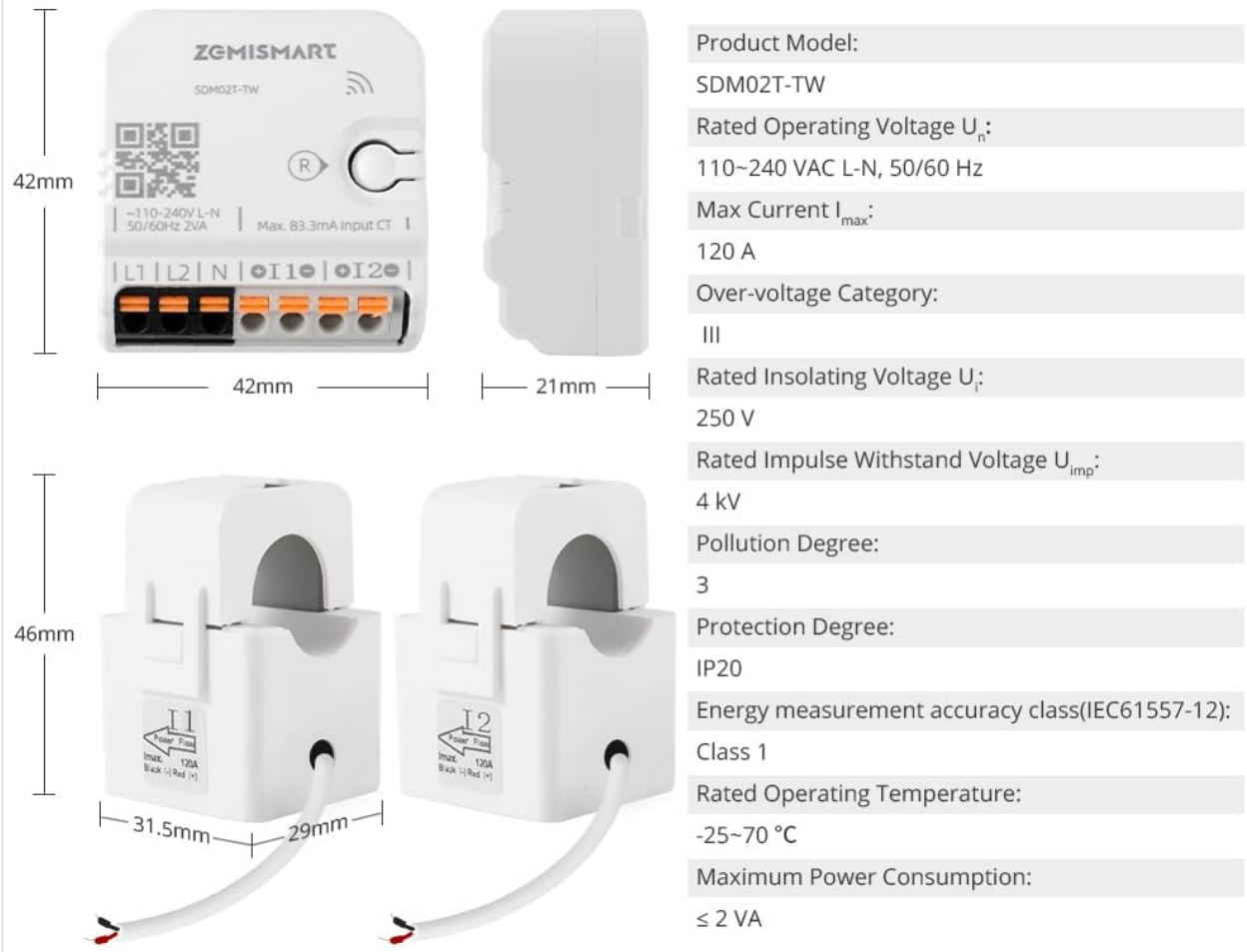
Image 7.1: This image provides a detailed overview of the product parameters and dimensions for the Blindsmart Smart Home Energy Monitor, model SDM02T-TW. It includes measurements for the monitoring module and the split-core CTs, along with electrical specifications such as rated operating voltage, max current, energy measurement accuracy, and operating temperature.
